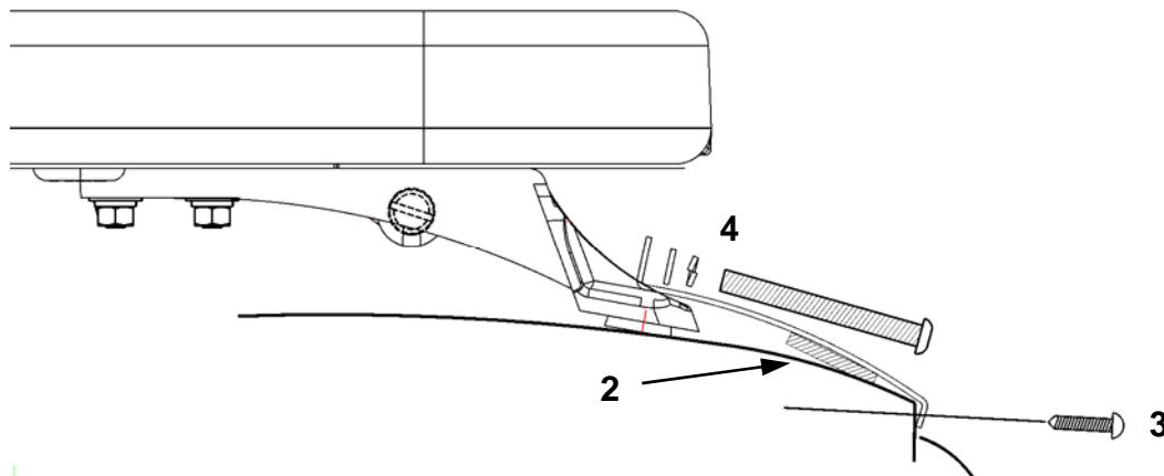
2. Mount the enclosed adhesive backed foam pad on the underside of the hook mount to protect the finish of the vehicle and to help reduce noise from excess vibration.
