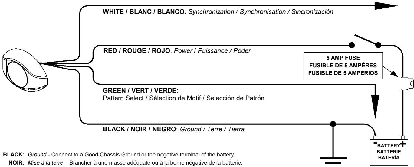
**BLACK:** Ground - Connect to a Good Chassis Ground or the negative terminal of the battery.
