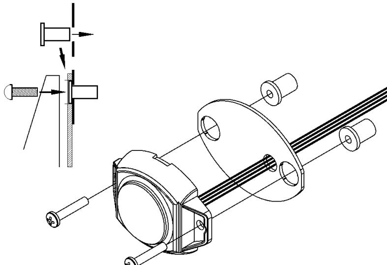
3. Push the well nuts through the holes until the lip rests on the surface.
