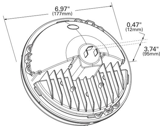
Upgrade to bright, efficient LED lighting with Grote's 7" LED Sealed Beam Headlight – a direct replacement for 7" halogen headlights.
